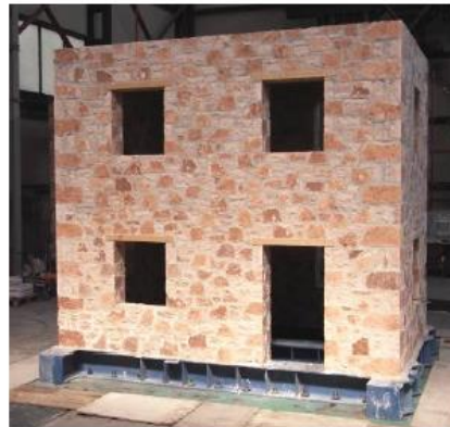
Fig. 1 a) Typical plan; b) The two storey building model on the shaking table
