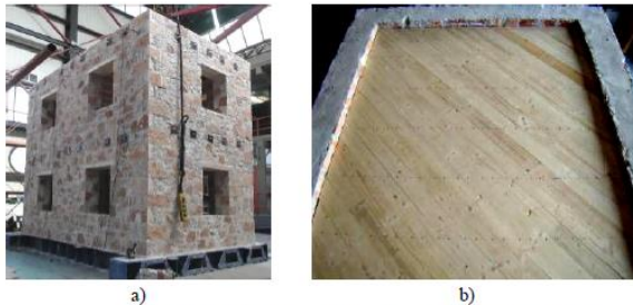
Fig. 6 Strengthened model a) general view and b) view from the top
