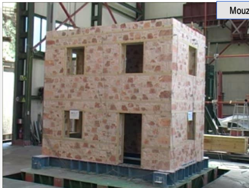
Fig. 1 Typical plan and picture of timber-laced specimen
