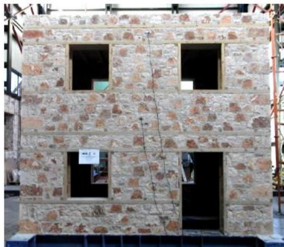
Fig. 1 Typical plan and picture of timber-laced specimen
