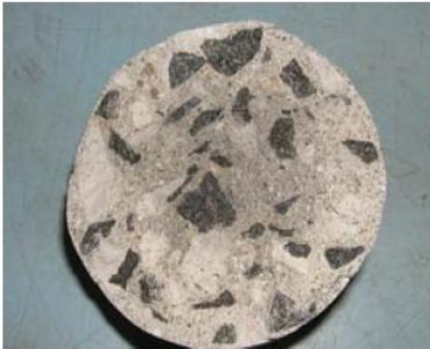
Concrete exposed to CO 2 (accelerated test)
