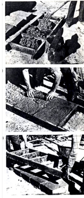
(b) Fig. 5.2. The use of straw in adobe blocks. Photograph (a) shows the appearance of adobe blocks one with too much straw and the other with the correct quantity of straw. Photograph (b) shows the crack-distributing effect of straw. Both the blocks were made from the same heavy clay, but the one without straw has cracked into two pieces.
