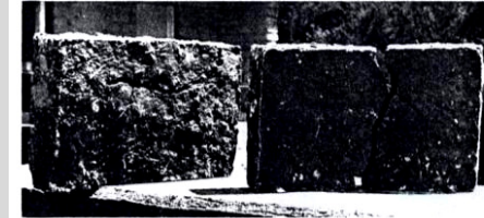
(b) Fig. 5.2. The use of straw in adobe blocks. Photograph (a) shows the appearance of adobe blocks one with too much straw and the other with the correct quantity of straw. Photograph (b) shows the crack-distributing effect of straw. Both the blocks were made from the same heavy clay, but the one without straw has cracked into two pieces.
