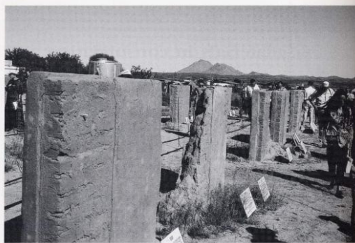
Figure 7.1 Work of the Getty Institute at Fort Lauderdale, New Mexico, 1990. Test panels set up in the open to provide data on modifications to earths in weathering, together with control panels, immediately adjacent. An important aspect of this research has been the sustained trialing of wide ranges of materials. For the first time on a large scale and with consistent techniques earth as a basic building material has been exposed to careful monitoring of its behaviour in scientifically prepared and supervised conditions. Only a sample of the trial series can be seen in these pictures.
