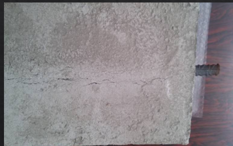
Correlation of Surface Cracks of Concrete due to Corrosion and Bond Strength (between Steel Bar and Concrete) Charis Apostolopoulos, K.Koulouris, Alk. Apostolopoulos, Journal Advances in Civil Engineering, 2019.
