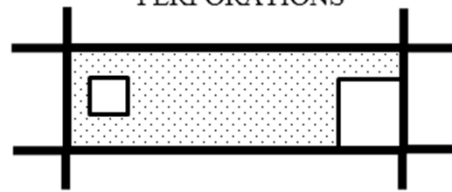
TWO BIG OPENINGS ADJACENT TO THE RC COLUMNS
